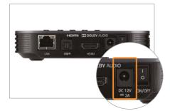
Plug the power adapter into the back.
