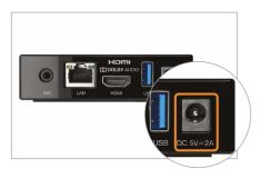
Plug the power adapter into the back.
