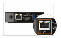
Plug the LAN cable into the back to connect the Internet.
